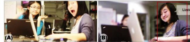
**Figure 2:** Gesture activated privacy demonstrated by a) the actual scenario captured by an ordinary camera b) live video stream as seen by remote viewer. Red box demonstrates privacy zone activated by right occupant with frozen pixels.
